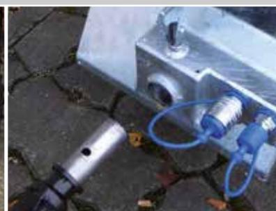
Hitch system and double-acting hydraulic connector (standard)
