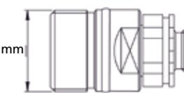
Size 1 = $\varnothing$ M 24x2<br>Size 3 = $\varnothing$ M 36x2<br>Size 4 = $\varnothing$ M 42x2<br>Size 5 = $\varnothing$ M 48x3 |
