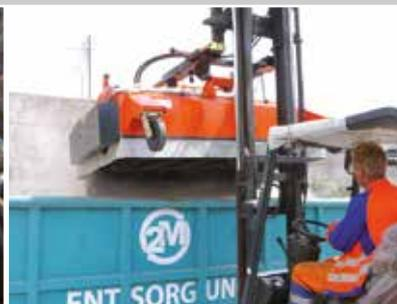
Hopper incl. hydraulic tip (standard)
