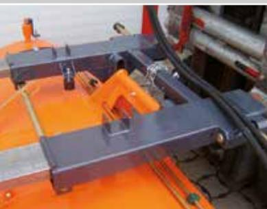
Hitch system with 3D levelling (standard)
