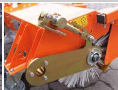
Broom adjustment via spindle
