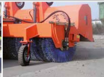
Easy brush adjustment by adjusting-lever system
