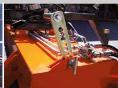
Adjusting-lever system with optimized sweeping-angle
