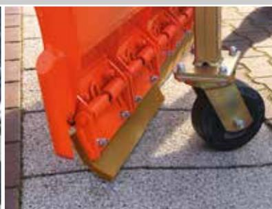
PU coated (standard) anti-icing spring flap segments
