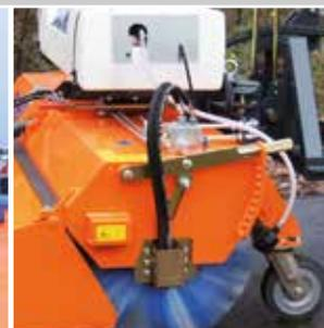
Adjusting-lever system with optimized sweeping-angle
